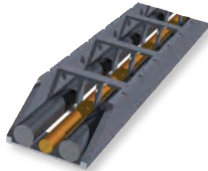
Use dividers horizontally and vertically to separate the track into separate cavities. Install just one cable per separated cavity. If absolutely necessary two small, or a small and a large cable can share a cavity.
