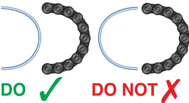
If possible the weight should be installed evenly within the cable track. Heavy cables should be installed on the outer edges, and lighter control and signal cables on the inside.
