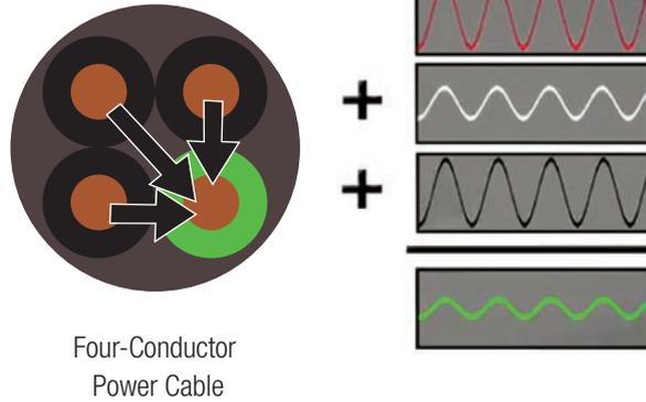
On the four-conductor cable shown above, the current flowing in the earth conductor is due to the differing voltages induced on the earth conductor, caused by the distance from each phase conductor to the earth conductor. This distance directly affects the capacitance between the different phase and earth conductors.
